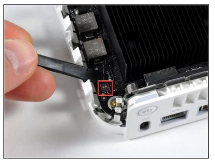
Use the flat end of a spudger to pry the power button cable connector up off the logic board.
