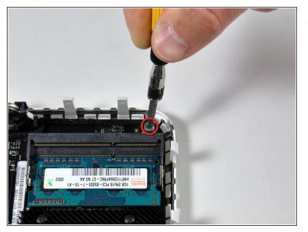
Remove the single T10 Torx lug next to the RAM sockets on the logic board.
