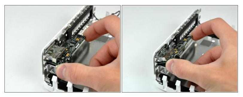
• Lift the audio board by its free edge and pull it away from the port side of the mini.
