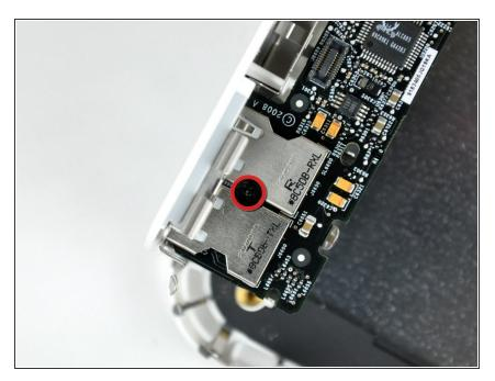
Remove the single Phillips screw between the headphone and microphone jacks on the audio board.
