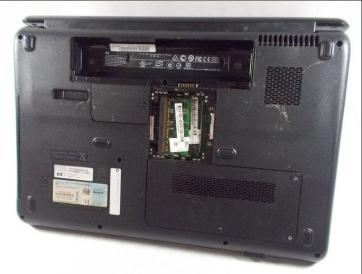
• Lift up on the RAM cover and remove it to reveal RAM sticks.
