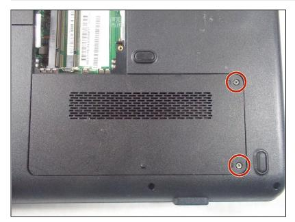
• Remove two 1.2 mm Philips#01 screws.
