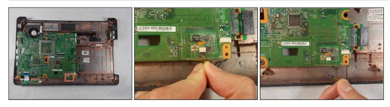
Disconnect the wire connected to motherboard by gently pulling downwards.
