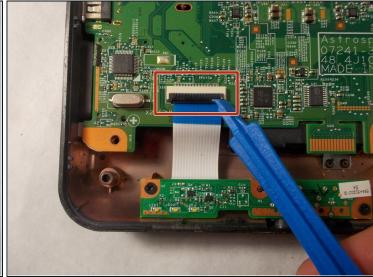
• Gently disconnect the ribbon cable using an opening tool.
