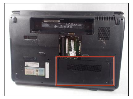
With the battery and RAM removed, locate the hard drive access panel.
