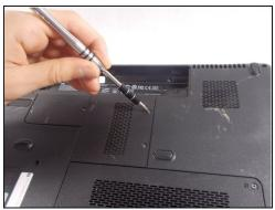
• Remove the two screws holding down the RAM access door with a Phillips #1 screwdriver.
