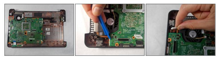
Disconnect the wire connected to the motherboard using an opening tool.
