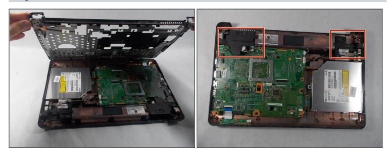
• lift up the casing and remove to reveal the speakers.
