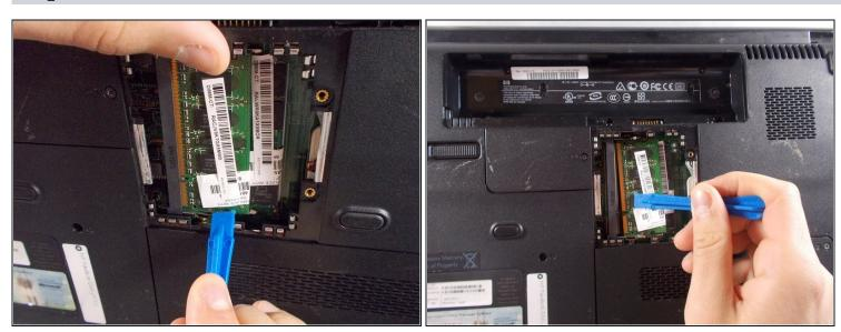
• Gently pull apart the two metal tabs located on both sides of the stick of RAM.
