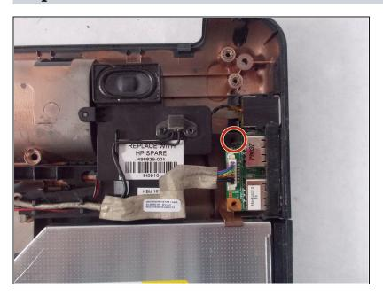
Remove highlighted 1.2 mm Philips #00 screw from right speaker.
