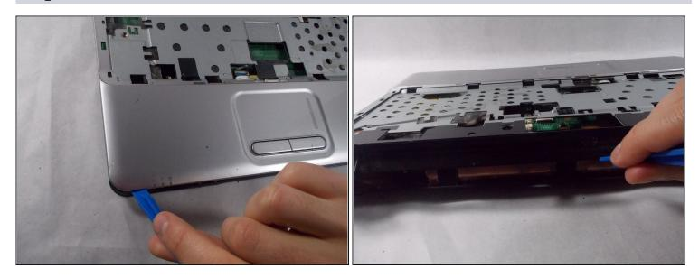
• Using a spudger unclip the casing around all corners and edges.
