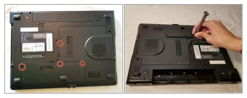
• Using the Phillips #1 screwdriver, remove the four 6mm screws on the back of the laptop.
