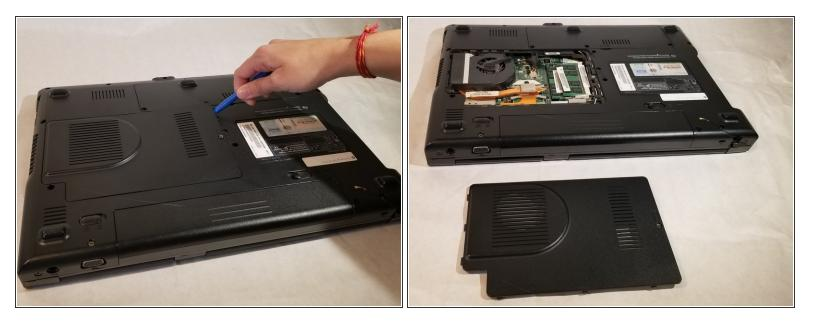
Insert the plastic prying tool and pry the back panel off starting at an edge and moving your way around it.
