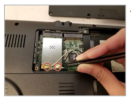
Use the tweezers to remove the two connecting wires.
