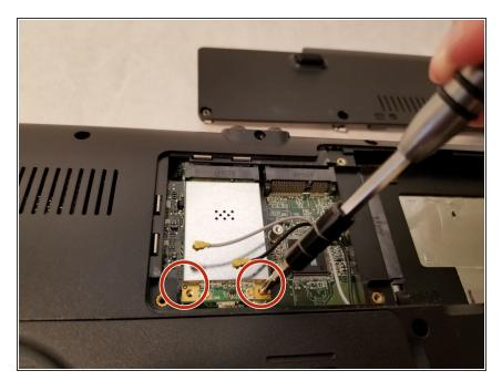
Using the Phillips #1 screwdriver, remove the two 2.5mm screws holding down the card.
