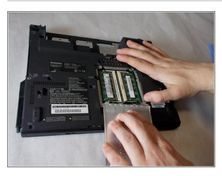
Now with the loosened screws, you can easily pull back the metal compartment cover to get to where RAM is stored.
