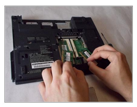
After opening up the compartment, you simply pull out the two RAM units and replace them with the new RAM.
