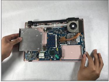
• Slide your finger from the right of the optical disc and pull the optical disc from right to left.
