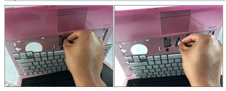
• Disconnect the keyboard by pulling the connection wire in the opposite direction of where it's connected.
