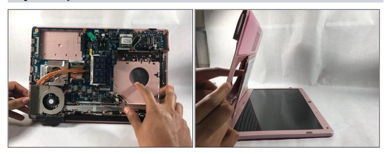
• Push keyboard out from the hole located in the optical drives original location.
