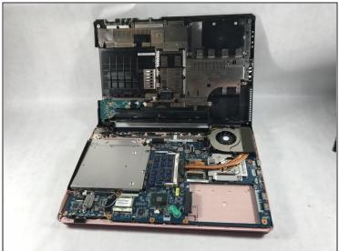
• Lift the backplate from bottom right and left corner and remove it from the laptop.
