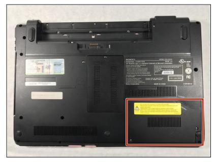
• The hard drive panel is located in the bottom right corner of the device.
