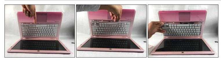
• Remove the keyboard cover by gently pulling along the sides until it is removed completely.
