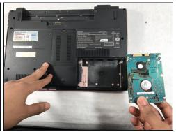
• Detach the hard drive by disconnecting it from the motherboard, pulling it gently from left to right.
