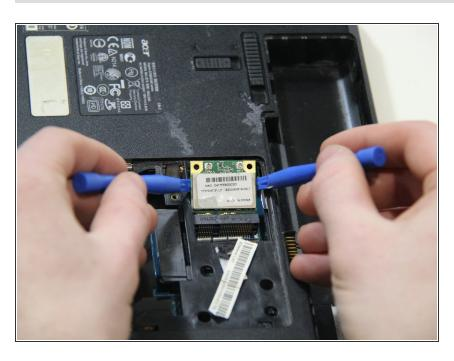
Carefully remove the module from the system, using plastic opening tools.
