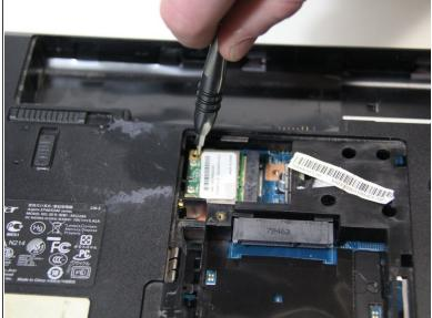
• Remove one M2 x L4 screw, which is securing the WLAN Module.
