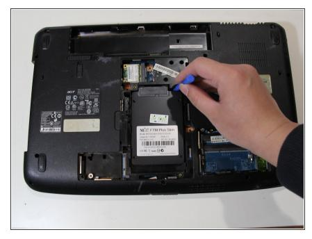
Using an opening tool or your hands, slide the hard drive out of its connector.
