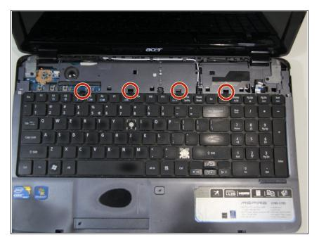
These latches must be released in order for the keyboard to be removed.
