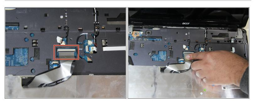
Using your hands, open the latch holding the wire in place, and remove the keyboard.
