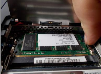
Pull the highlighted latches away from the sides of the RAM Stick to unlock it.
