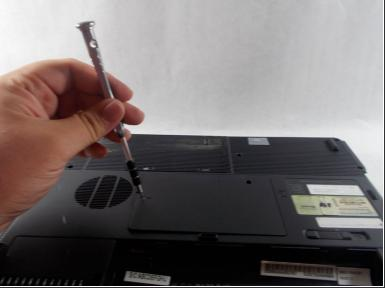
• Use the Phillips #0 Screwdriver to remove the 2 5mm screws.
