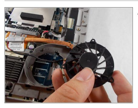
Remove the cooling fan, alongside its wire, from the fan's casing.
