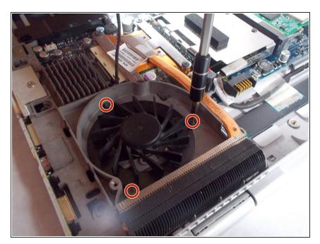
Use the Phillips #00 screwdriver on the three 4mm #00 screws affixing the fan to the laptop.
