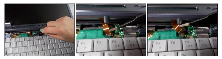
• Use the <u>tweezers</u> to disconnect the ribbon cable from the motherboard.
