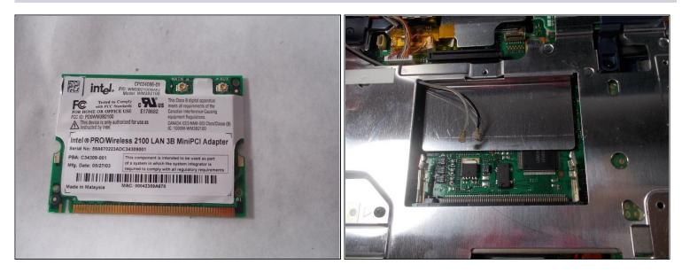
• Take out the Adapter and carefully pull the wires out from the metal casing.
