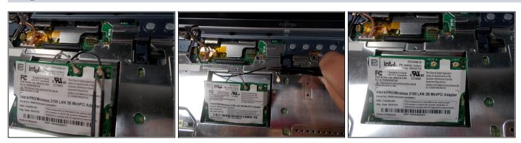
• Use <u>tweezers</u> to remove the wires from the Adapter.
