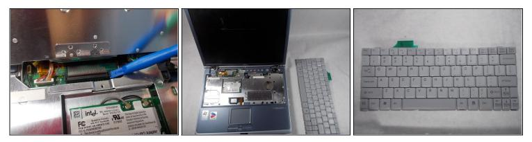
• Use a plastic opening tool to release the ribbon cable from the motherboard.
