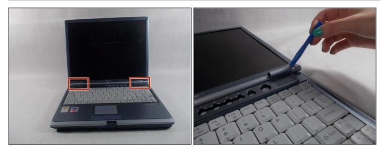
• Use a plastic opening tool to lift the back of the hinge cover on the left and right sides of the computer.
