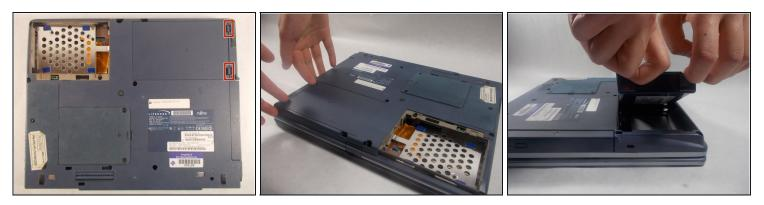
To prevent injury, make sure the laptop is unplugged and turned off before removing the battery.
