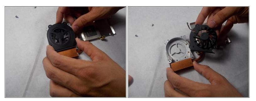
Remove the fan from its metal protective cover.
