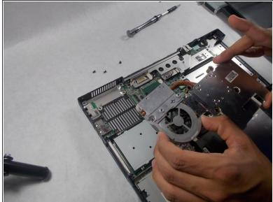
Now that its not fixed to the laptop's interior, remove the entire fan assembly from the laptop.
