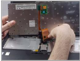
Lift the keyboard and remove the keyboard ribbon cable from the laptop
