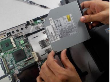
Remove the optical drive from the laptop's interior.
