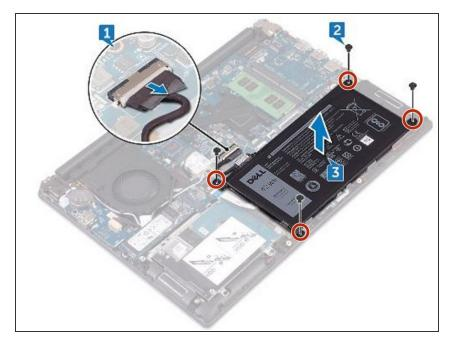
Align the screw holes on the NEW battery with the screw holes on the palm rest and keyboard assembly.
