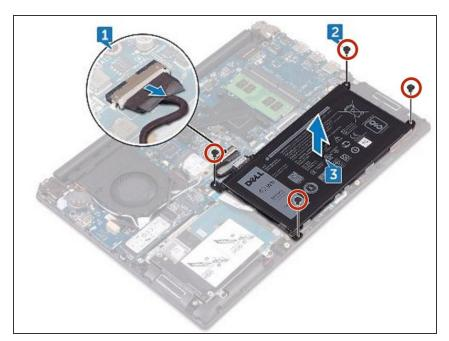
Replace the four screws (M2x3) that secure the battery to the palm rest and keyboard assembly.
