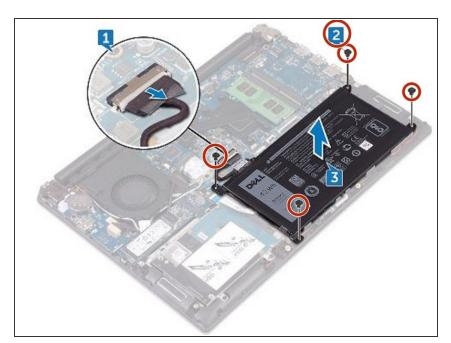
Remove the four screws (M2x3) that secure the battery to the palm rest and keyboard assembly.
