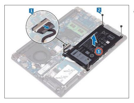
• Lift the battery off the palm rest and keyboard assembly.
