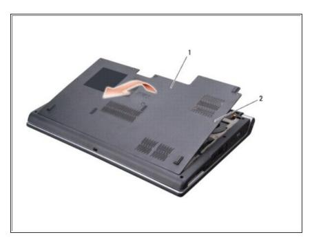
Loosen the eight captive screws on the base cover and lift the cover off the computer at an angle as shown in the figure.
