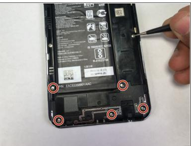
Remove the twelve 2.5mm Phillips #0 screws from the back of the phone.
