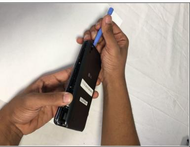
Insert a plastic opening tool above the AUX jack and slide it around the perimeter to pop the back cover off.
