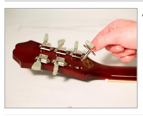
The tuner should come right out of the back of the head of the guitar.
