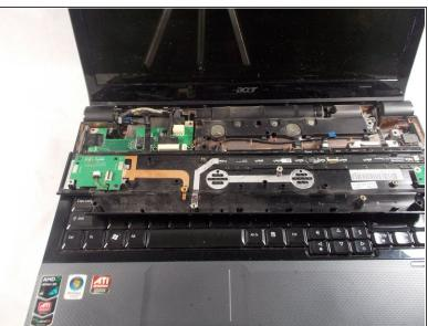
Lift the top panel up from the back, turning it over forward.
