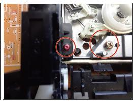
Unscrew all of these screws to remove the main plate
