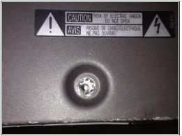
The first step is to unscrew both screws on both sides of the VCR
