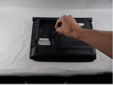
Using a Phillips #1 screwdriver, remove the 7mm screw holding the drive.
