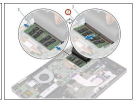
Use your fingertips to carefully spread apart the securing-clips on each end of the memory-module slot until the memory module pops up.
