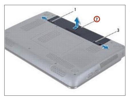
Slide the **NEW** battery into the battery bay, until it clicks into place.
