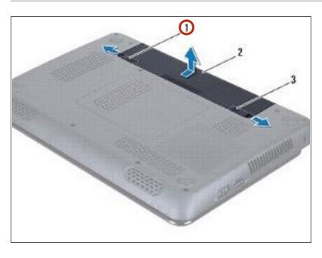
Slide the battery release latch to the side.
