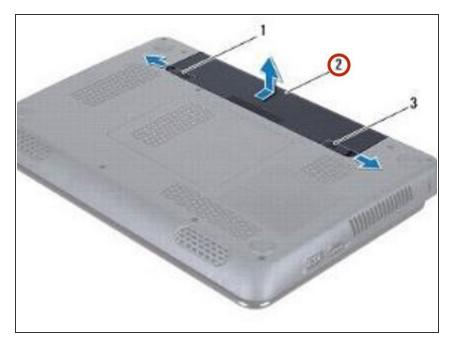
Slide and lift the battery out of the battery bay.
