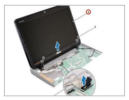
Lift the display assembly off the computer.
