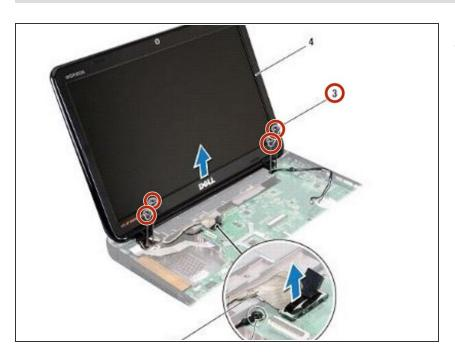
In sequential order (indicated on the display hinge), remove the four screws that secure the display assembly to the computer base.
