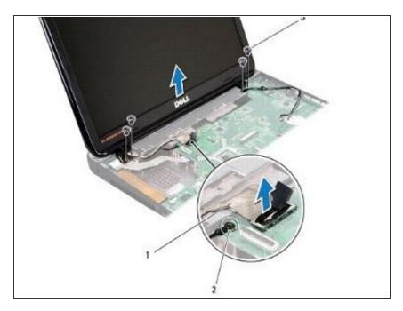
In sequential order (indicated on the display hinge), replace the four screws that secure the display assembly to the computer base.
