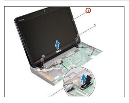
Place the **NEW** display assembly in position.
