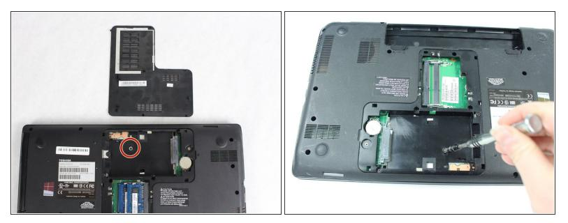
• Using the JIS #000 screwdriver, remove the .5mm screw.
