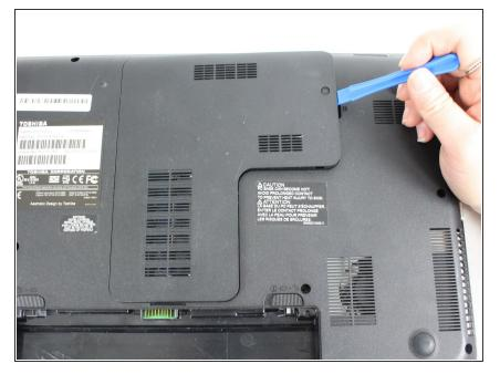
Remove the panel with the plastic opening tool. Make sure you lift it on all four sides.
