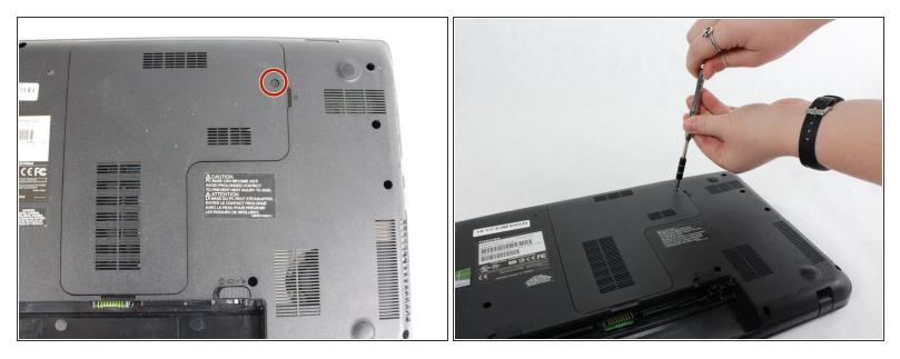
Remove this screw with a JIS #000 screwdriver.
