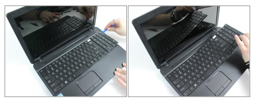
• Use the plastic opening tool to remove the keyboard from the laptop.
