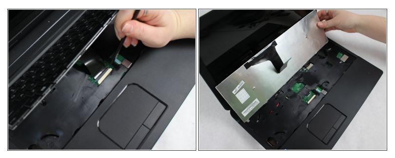
• Once keyboard is popped out, use a nylon spudger to undo the ribbon or flap that attaches the back of the keyboard to the inside base of the laptop.
