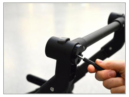
• Remove the bottom part of the cylinder. You can use your screwdriver to pull it out.
