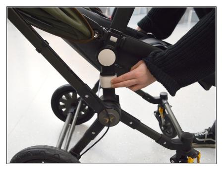
• Push both the white square buttons under the seat at the same time, to remove the seat from the frame.
