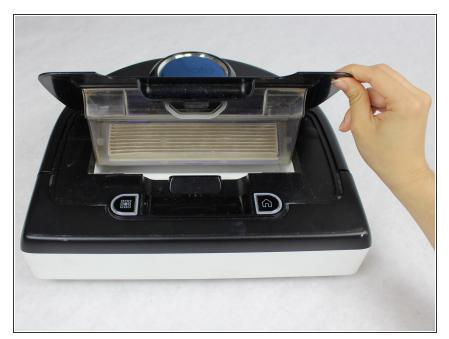
Grasp the top latch of the filter cover and gently lift up to reveal the air filter.
