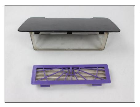
Once the filter has been completely removed, you may clean or replace the filter.
