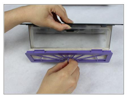
After you take out the holster from the robot, pull the tab to remove the filter.
