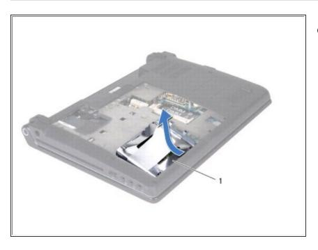
Tilt the hard drive by 45-degrees and lift it out of the computer base.
