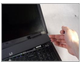
Use the Plastic Opening Tools to pry off the tab located on the right side of the top face plate.
