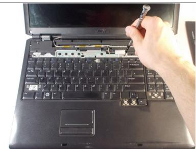
Remove the four 3mm Phillips #0 screws.
