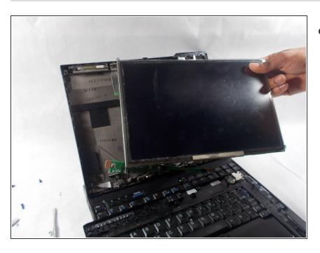
Once all screws are removed, remove the LCD Display but gently peeling back line a sticker
