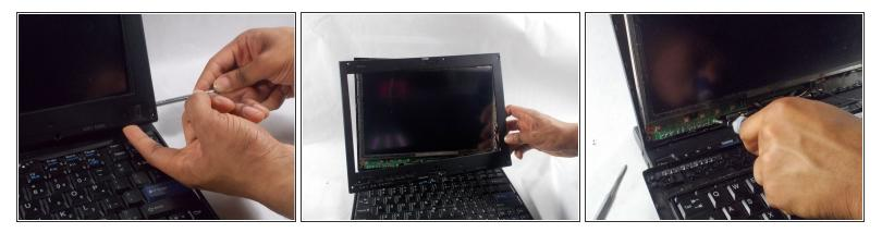
• Gently pry the LCD cover with a flat head screwdriver, and pivot it over the signal cable near the LCD hinges. Pivot over all four corners
