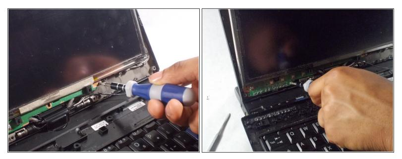
Continue to remove screens in front of the LCD cover, make sure all screws in the front are removed
