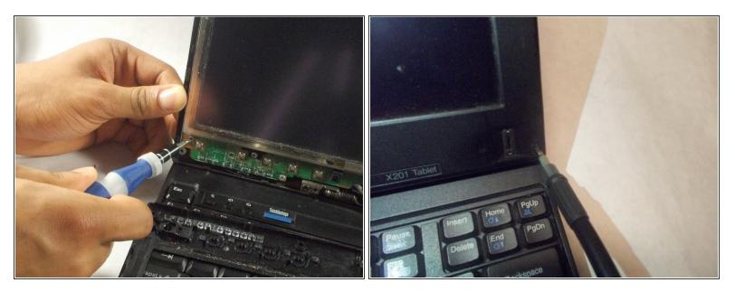
• Unscrew the screws on the front of the LCD screen
