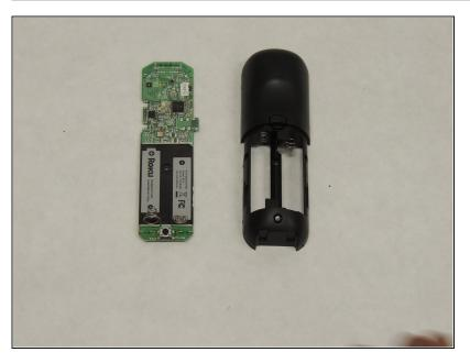
The contacts should be present with one set being in the bottom of the remote casing and the other set being on the underside of the motherboard for the remote.
