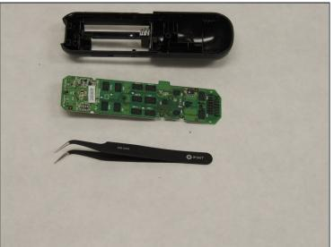
• Using tweezers, remove the motherboard from the remote.
