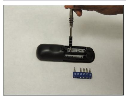
Remove the screw using a Phillips #00 screwdriver.
