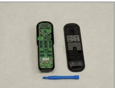
• Remove the face of the remote with the plastic opening tool.
