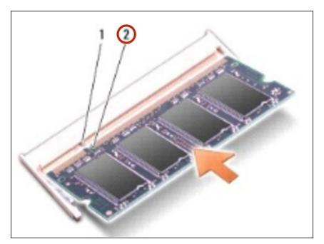
Align the notch in the module edge connector with the tab in the connector slot.
