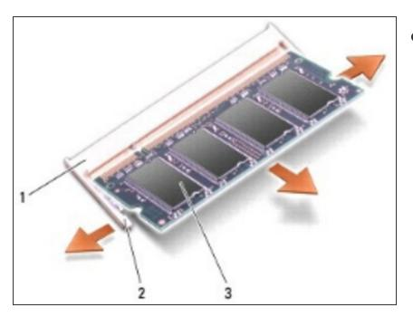
• Remove the module from the connector.
