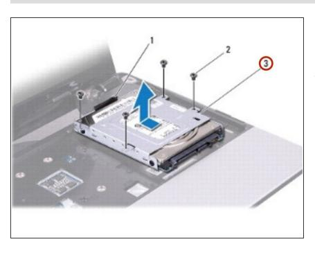
Slide the hard drive assembly to disconnect it from the system board connector.
