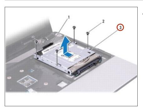
Place the hard drive assembly in the computer base.
