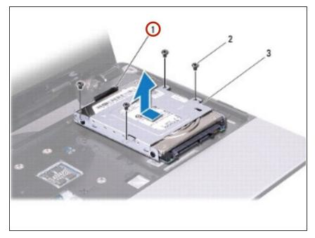
Pull the black pull-tab and lift the hard drive assembly out of the computer base.
