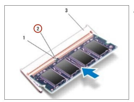
Align the notch in the NEW memory module with the tab in the memory module connector.
