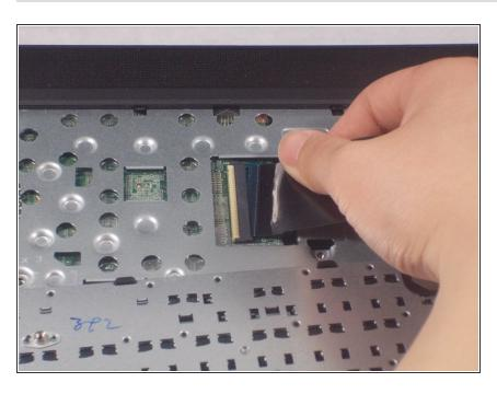
Disconnect the connected cable from the mainboard.
