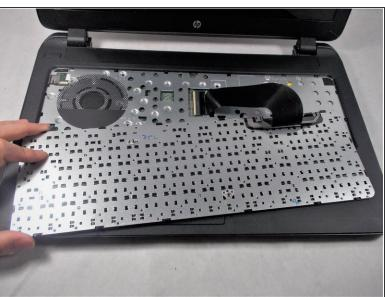
Pry the keyboard out of the laptop gently and flip the keyboard around.
