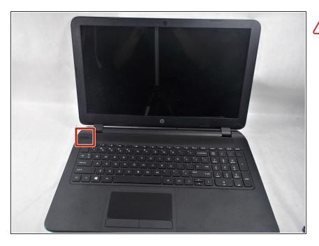
Turn off the computer. If you are unsure whether the computer is off or in Hibernation, turn the computer on, and then shut it down through the operating system.
