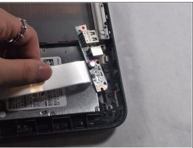
Use a Phillips #0 screwdriver to remove the screw that holds the USB drive in the bottom right corner near the hard drive. Once removed, lift the USB drive off of the hard drive.
