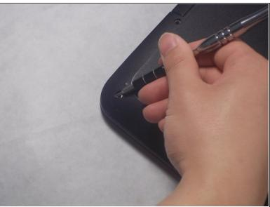
Remove the twelve screws from the bottom of the laptop with the Philips #0 Screwdriver.
