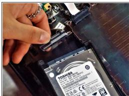
• Lift the hard drive from the device and unconnect the cord attached to it.
