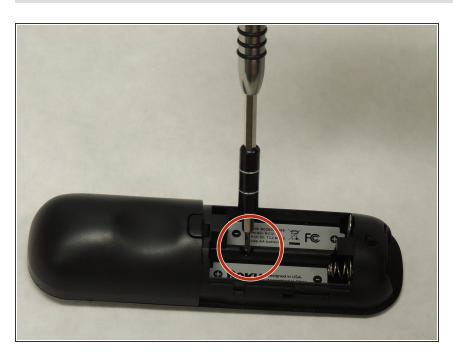
• Use a Phillips #00 screwdriver to remove the 1.5 mm wide screw.
