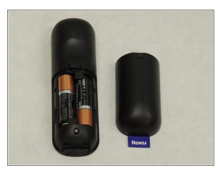
• Remove the battery cover to expose the battery compartment.
