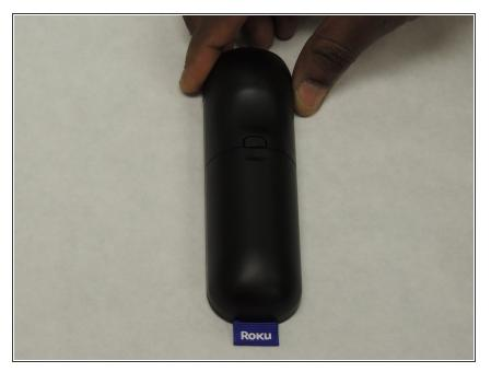
• Place the remote so that the battery cover is facing upwards.
