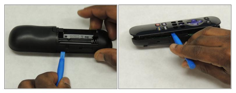
• Use a plastic opening tool to gently pry apart the plastic enclosure. Make sure you create a large enough gap before you attempt to separate the two pieces.
