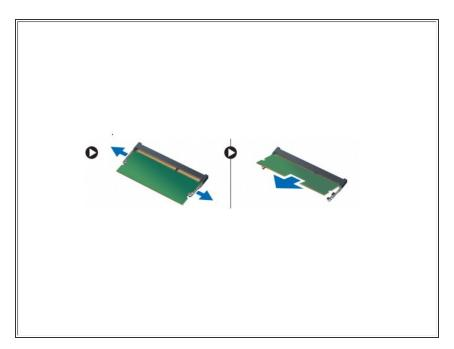
Pry the retention clips away from the memory until it pops up. Lift the memory and remove it from the computer.
