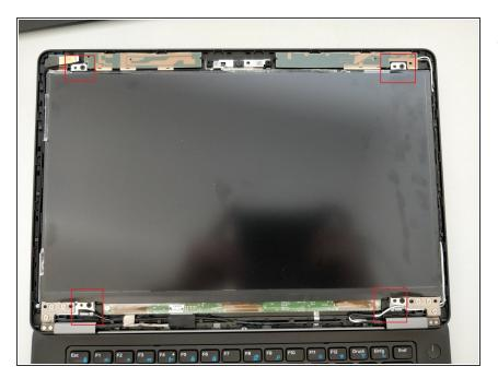
Remove the 4 Philips screws securing the panel.
