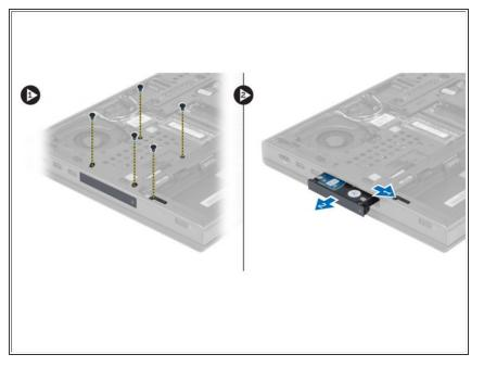
• Remove the screws that secure the hard drive to the computer. Slide the hard -drive latch to the unlock position and pull out the hard drive from the computer.
