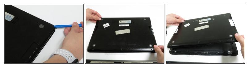
• Find an opening on the back of the laptop. Use the plastic prying tool to help pry open the back panel of the laptop.
