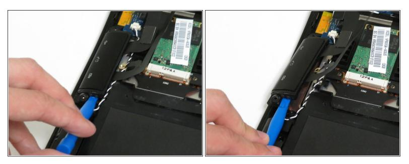
Find an opening on the side of the port and pry the USB and AUX port out of the laptop with the prying tool.
