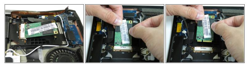
(i) After removing the screws, your card should angle upward making for an easier removal.
