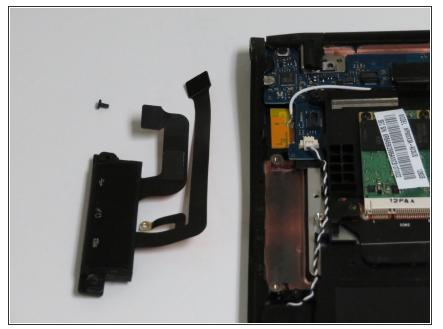
• Remove and place the port outside of the laptop. You are free to install your new USB and HDMI ports.
