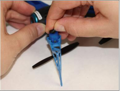
• With the camera facing you, firmly grasp the small black rubber button like foot and squeeze it.
