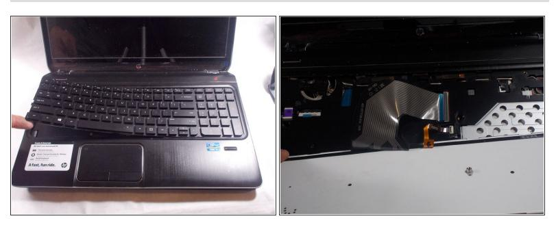
Carefully pull up on the key board there will be 2 ribbon strips holding it attached to the key board
