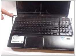
Pry off the keyboard retainer slowly working your way around the board to prevent damage
