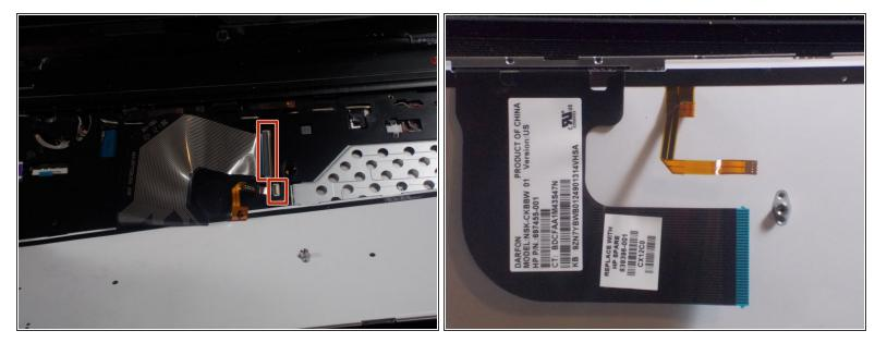
Pull up on the two grey tabs that hold the ribbon cable into the connector. Then remove the keyboard. To reassemble your device, follow these instructions in reverse order.
