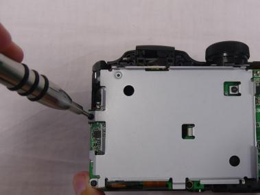
Remove three 4mm JIS #000 screws from the metal housing plate.
