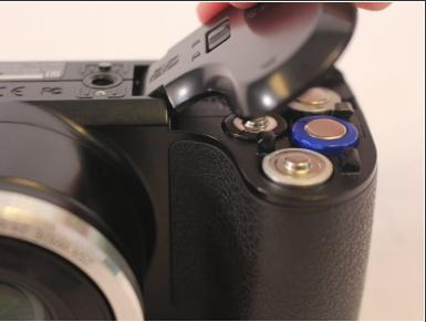
Press down on the battery cover and slide outwards to open.
