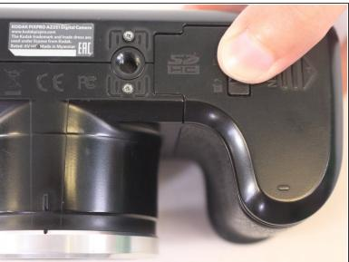
Slide switch to open lock position.
