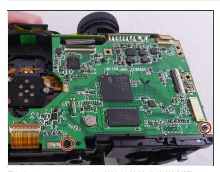
Remove the two 4mm JIS #000 screws from the motherboard.
