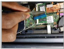
There will be a metallic film attached to the keyboard from the motherboard. A black latch runs along the film keeping it in place. Lift the latch and detach the film; remove it to fully remove the keyboard.
