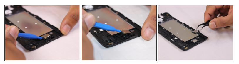
Use a plastic opening tool to pry up the speaker.
