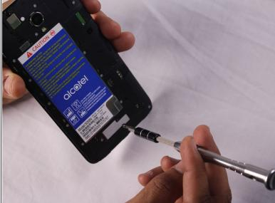
Remove the seventeen Phillips #000 screws from the mid-frame.
