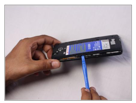
Pry off the mid-frame using a plastic opening tool, working your way around the perimeter.
