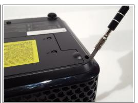
Start by removing the two screws on the bottom of the device as shown.
