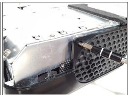
Remove the screws from the case located around the device.
