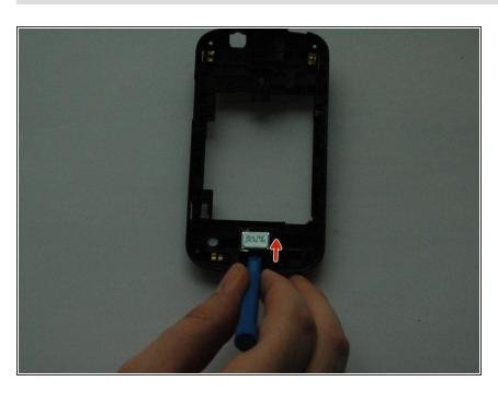
Using the plastic opening tool, gently lift the speaker out of the back case.
