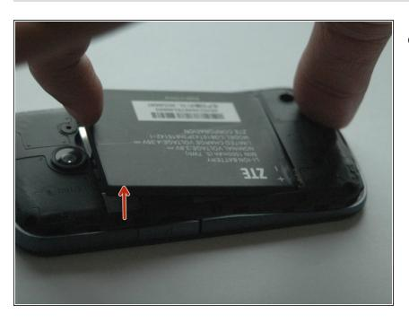
Remove the battery by inserting your fingernail at the top of the battery and lift up.
