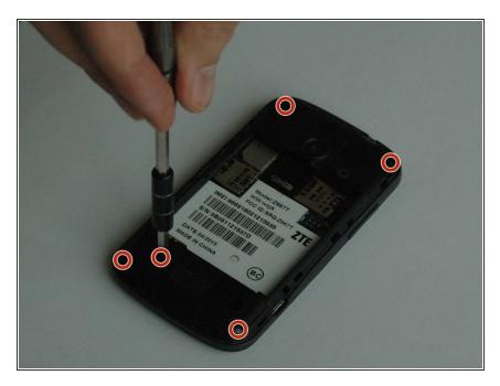
Using a Phillips #000 screwdriver, remove the five screws located on the back case.
