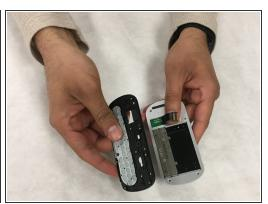
There are six 2mm screws that connect the keypad piece to the other side of the phone. Using a Phillips #000 screwdriver, remove those screws and separate the two sides of the phone.
