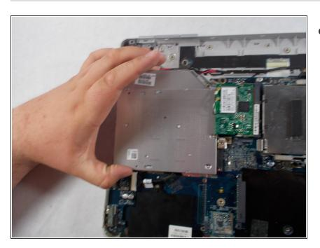
Gently remove the disk drive from its socket.
